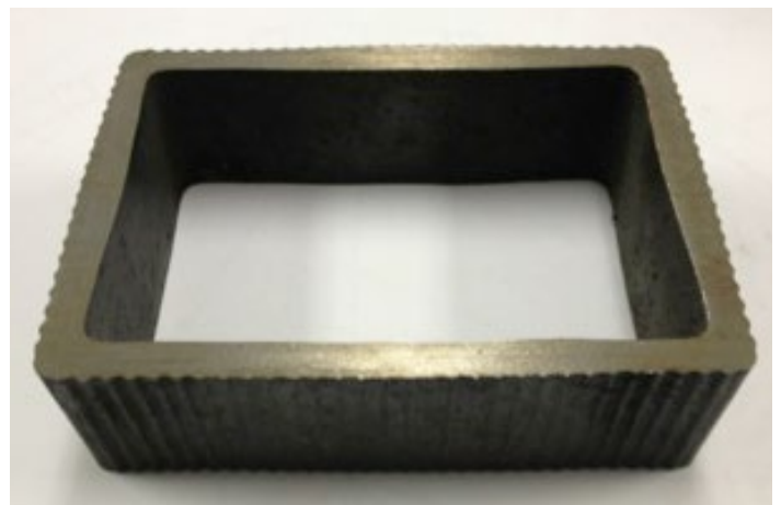
Fig. 9 Breakout shell from 0.45% carbon steel cast with WAVE mould.
